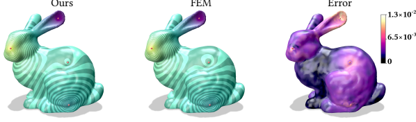
Fig. 4. Solving screened Poisson equation. As the prescribed sources diffuse across the entire surface, our neural approach (left) achieves a low approximation error compared to standard FEM-based methods (middle). The pointwise error (right) is computed as |u_i^{\text{ours}} - u_i^{\text{fem}}| / \|u^{\text{fem}}\|_{\infty} .
